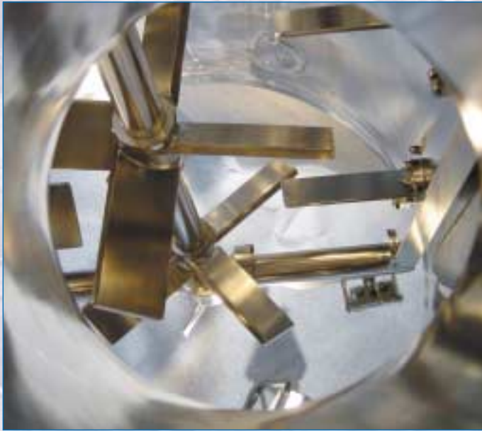
Mixer inside the vessel
