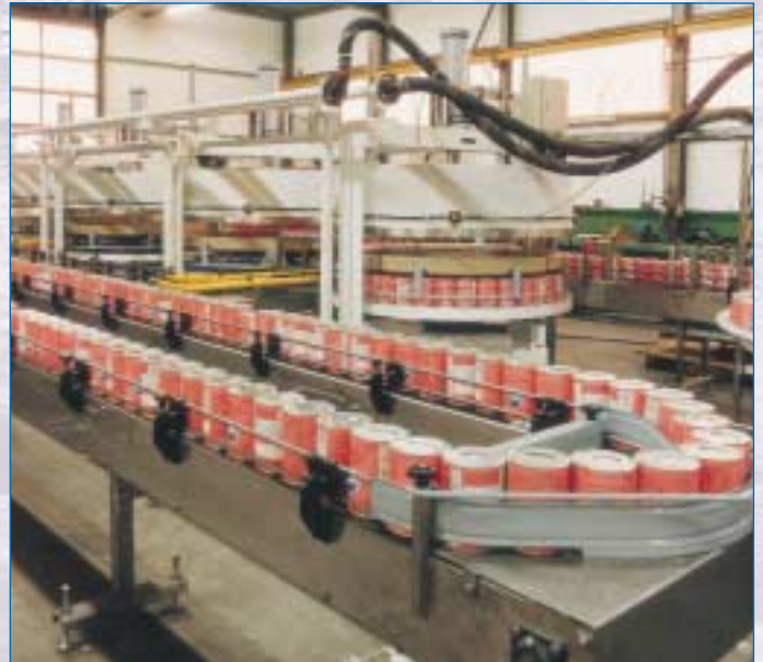
Vacuumizing & Gassing unit
