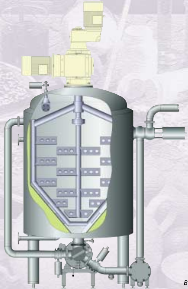
Terlotherm scraped surface heat exchanger
